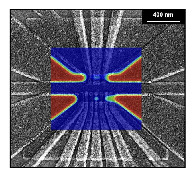
A scanning electron microscope (SEM) image of a device lithographically identical to the one measured shows the gate electrode layout in the active region.
