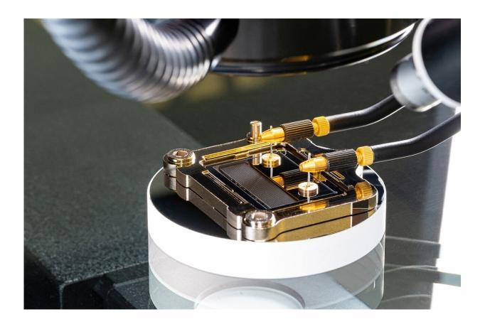
Double slit module during precision assembly in the coordinate measuring machine. Credit: Fraunhofer-Gesellschaft
