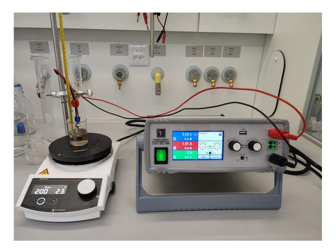
Setup of an electrochemical oxidation test: diamond electrodes in sulfuric acid arsenic(III) oxide solution. Credit: Fraunhofer IWKS
