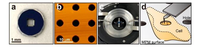
Figure 1. A new technique for observing living cell membranes for AFM using porous silicon nitride membrane (MPM). (a) The appearance of MPM. (b) The holes of MPM observed by AFM. (c) The MPM when set in the chamber for observation. (d) Schematic of AFM cell surface observation using MPM. Credit: Kanazawa University
