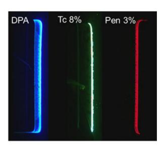
The design concept of molecular doping and electroluminescence images of three primary color light-emitting transistors. Credit: Qin Zhengsheng
