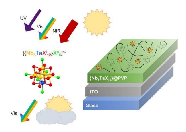
The nanoclusters are dispersed in a PVP matrix that is then coated on ITO glass to block NIR and UV rays while letting visible light pass through. Credit: Science and Technology of Advanced Materials
