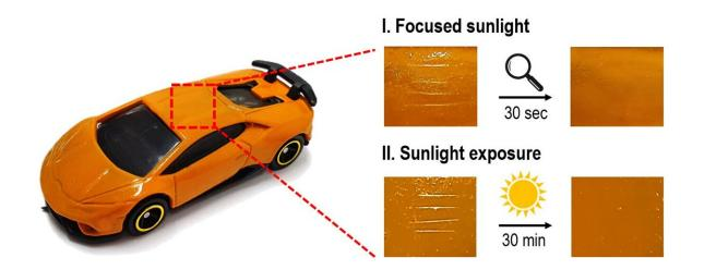
Self-healed surface of a model car after scratching when exposed to focused sunlight with a magnifying glass (upper) or to sunlight directly (down). Credit: Korea Research Institute of Chemical Technology (KRICT)
