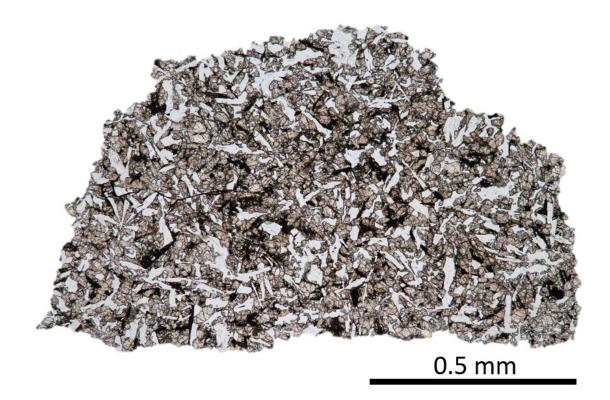
Thin section of NASA sample, LAP 02436, Lunar Mare Basalt containing indigenous noble gases. Image type: optical microscopy, plane-polarized light. Credit: ETH Zurich / Patrizia Will
