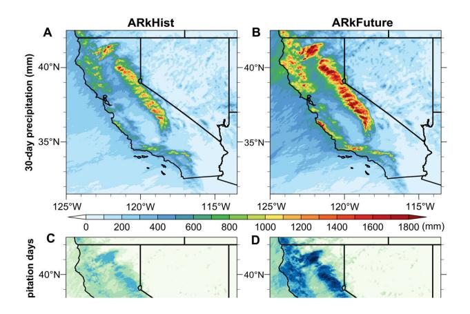
Precipitation associated with California megastorm scenarios.(**A** and **B**) Cumulative 30-day precipitation (mm) during ARkHist (A) and ARkFuture (B). (**C** and **D**) Cumulative number of heavy precipitation days (days with precipitation > 20 mm/day) during ARkHist (**C**) and ARkFuture (**D**). (**E** and **F**) Cumulative number of heavy precipitation hours (hours with precipitation >10 mm/hour) during ARkHist (**E**) and ARkFuture (**F**). (**G** and **H**) Time series
