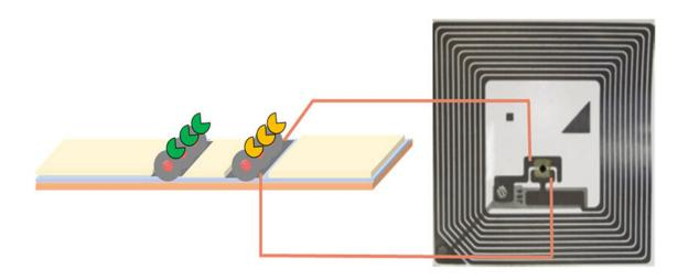
In this lateral flow assay, the paper that wicks the solution (left) has control and test lines that can be wired in parallel with the integrated circuit of an RFID device for wireless detection by a smartphone. Credit: Massachusetts Institute of Technology
