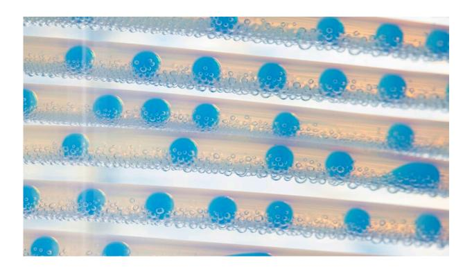
Assembly line: A different chemical mixture is created in each of the droplets within the "Tubular flow reactor"—under exactly the same boundary conditions. Credit: Empa
