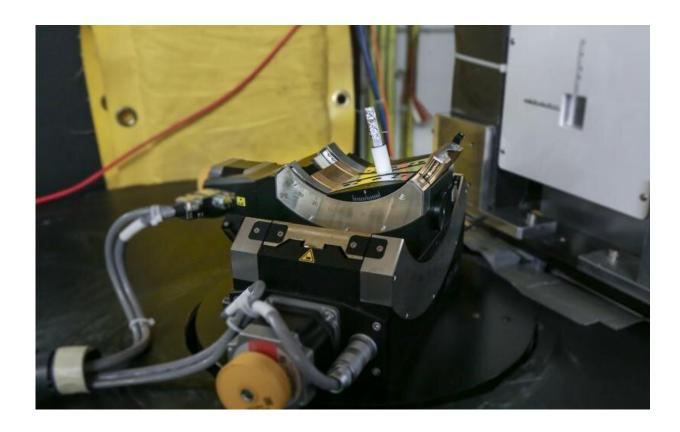
The AI-driven HyperCT platform has three primary points of articulation that can rotate a sample in almost any direction, eliminating the need for human intervention and significantly reducing lengthy experiment times. Credit: Genevieve Martin, ORNL/U.S. Dept. of Energy
