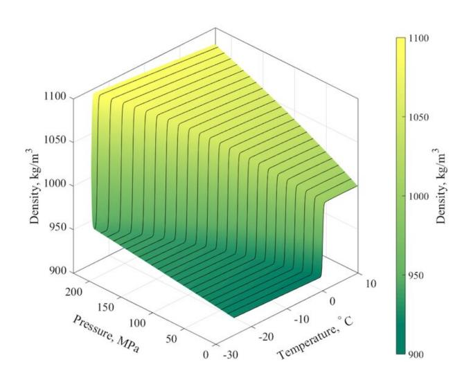
Density of water within the range of pressures and temperatures that the researchers investigated. Credit: Biothermal Technology Laboratory, Carnegie Mellon University
