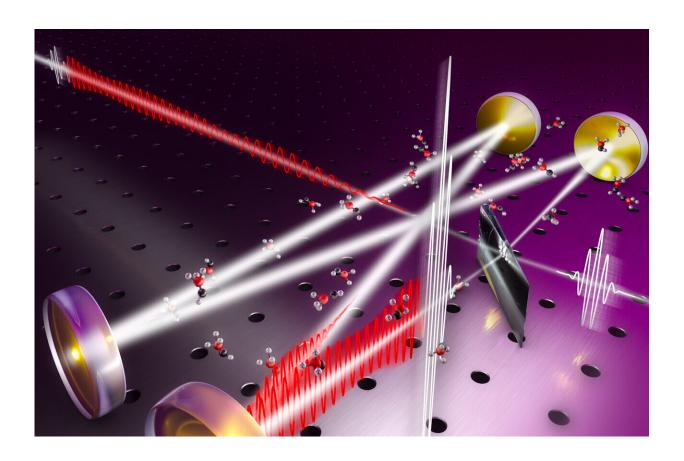
Enhancement of laser pulses (white) and molecular responses (red) in a passive optical resonator. Credit: Christian Hackenberger
