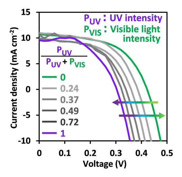
JV characteristics of a SbSI:Sb2S3 photovoltaic device under the simultaneous irradiation of ultraviolet (UV) and visible (VIS) light with varying intensity ratios. This figure is reproduced from the original paper (Figure2e). Credit: Ryosuke Nishikubo et al., *Advanced Functional Materials*, CC BY
