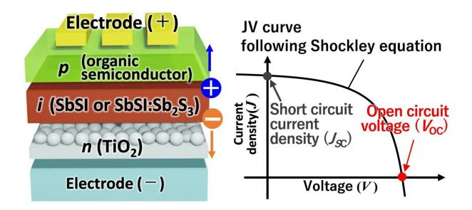
Device structure (left) and schematic of current density-voltage (JV) characteristics. This figure is reproduced from the original paper (Figure1a). Credit: Ryosuke Nishikubo
