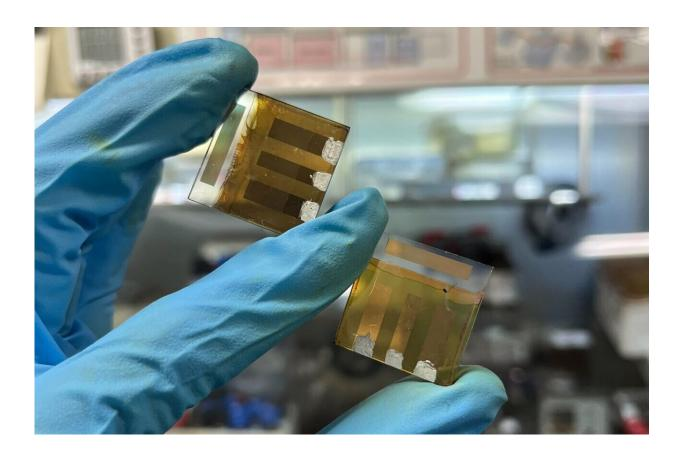
SbSI and SbSI:Sb<sub>2</sub>S<sub>3</sub> photovoltaic devices. Credit: Ryosuke Nishikubo
