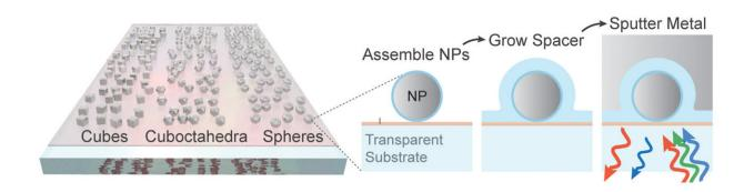
A new upside-down fabrication method for light-manipulating metamaterials envelops nanoparticles with a transparent spacing layer followed by a coating of metal. The way the metal coating envelops part of the nanoparticle while maintaining tight, nanometer tolerances allows for a much larger design space than was previously possible. Credit: Jon Stewart, Duke University
