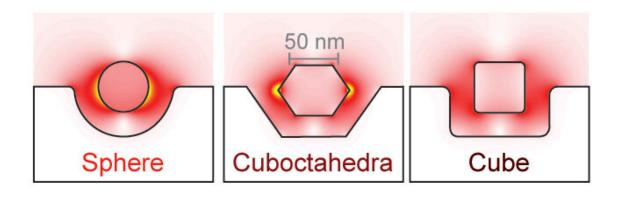
The new upside-down fabrication method allows researchers to use a wide variety of new nanoparticle shapes, such as spheres and cuboctahedra—a shape consisting of eight triangular faces and six square faces. Credit: Jon Stewart, Duke University
