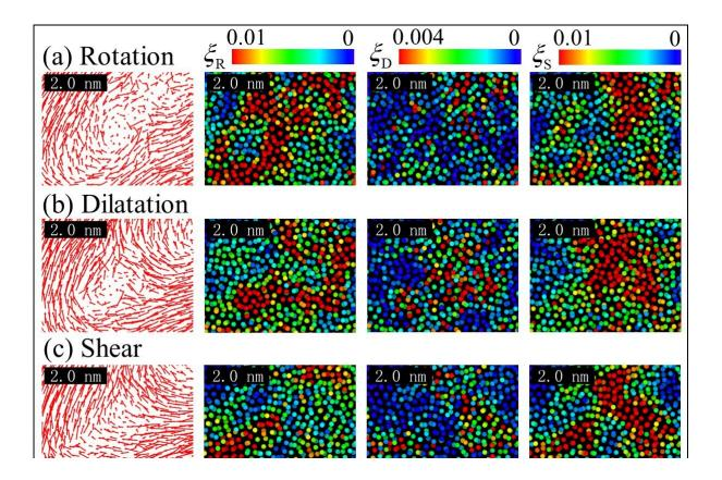
Quantitative characterizations of shear, dilatation and rotation motions in shear bands via the TTG model. Credit: IMCAS
