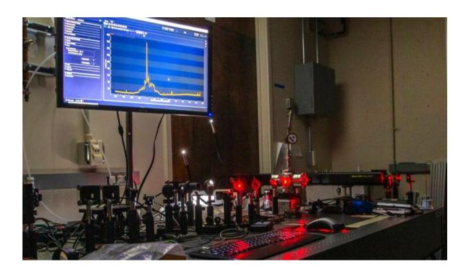
Shown on a large computer screen is a Raman spectrum of uranium oxide particulates formed inside the team's benchtop reaction chamber. The uranium oxide spectrum shown is for  $U_3O_8$ . Credit: Julie Russell/LLNL
