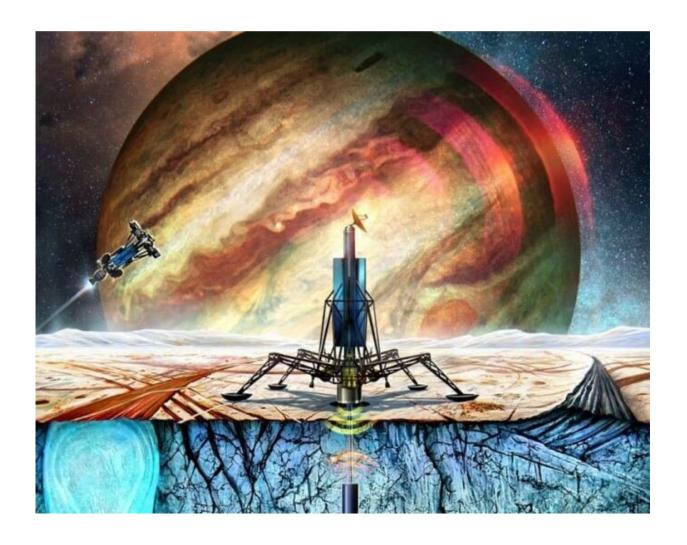
This illustration explains how the SWIM concept works. A lander sits on Europa's surface, and a cryobot tunnels its way through the ice while remaining data-tethered to the lander. The cryobot gathers data as it tunnels its way through the ice. Once into the ocean, the cryobot releases about four dozen small SWIMbots to gather data. Credit: NASA/JPL-Caltech
