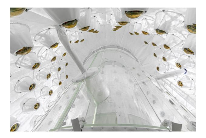
Looking up into the LZ Outer Detector, used to veto radioactivity that can mimic a dark matter signal. Credit: Matthew Kapust/Sanford Underground Research Facility
