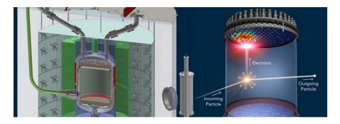
(Left) A schematic of the LZ detector. (Right) Illustration of LZ operation—particles interact in liquid xenon, releasing a flash of light and charge that are collected by photomultiplier tube arrays at top and bottom. Credit: Left schematic: LZ collaboration. Right image: LZ/SLAC
