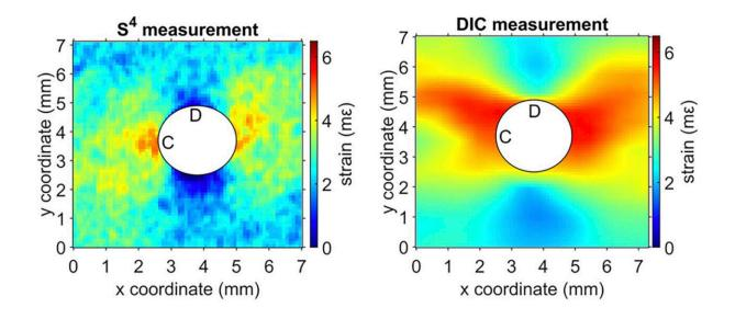
A comparison of measurements on an acrylic under strain shows Rice University's S4 system, left, gives a more detailed readout than standard digital image correlation (DIC) at right. Credit: Nagarajaiah and Weisman Research Groups / Rice University
