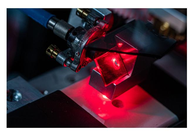
A Rice University lab tests material covered in strain-sensing smart skin. The multilayer coating contains carbon nanotubes that fluoresce when under strain, matching the strain experienced by the material underneath. Credit: Jeff Fitlow / Rice University
