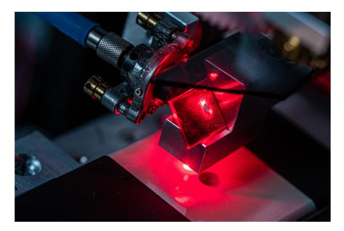
A Rice University lab tests material covered in strain-sensing smart skin. The multilayer coating contains carbon nanotubes that fluoresce when under strain, matching the strain experienced by the material underneath. Credit: Jeff Fitlow / Rice University
