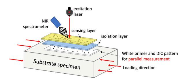
A three-layer smart skin on a structure can detect strain through the fluorescence of embedded carbon nanotubes, according to its inventors at Rice University. The skin can be painted or sprayed on buildings, bridges, aircraft and ships to provide a non-contact way to monitor the structural health of a structure. Credit: Nagarajaiah and Weisman Research Groups / Rice University
