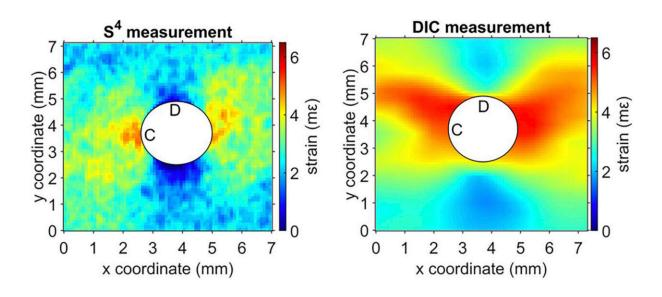
A comparison of measurements on an acrylic under strain shows Rice University's S4 system, left, gives a more detailed readout than standard digital image correlation (DIC) at right. Credit: Nagarajaiah and Weisman Research Groups / Rice University
