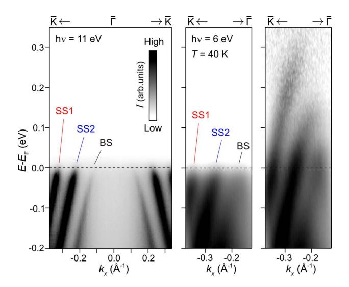
Left: Electronic structure of GeTe taken with 11 eV photons at BESSY-II, showing the band dispersions of bulk (BS) and surface Rashba states (SS1, SS2)
