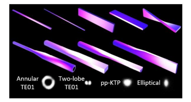
SPIM-WGs with varying cross-sections, enabling mode conversion. Credit: Bangshan Sun
