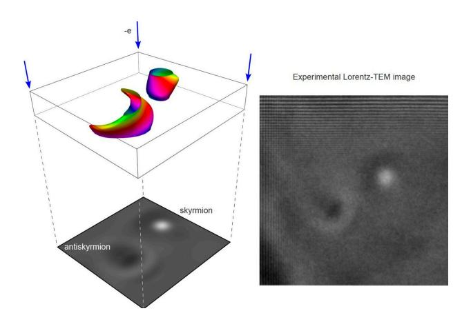
Left: Skyrmion-antiskyrmion pair predicted using micromagnetic simulations and a corresponding simulated Lorentz TEM image in the over-focus regime. The isosurfaces correspond to the positions of magnetization vectors lying in the plane of the film. The color indicates the direction of the magnetization vectors in the plane. Right: Experimental Lorentz TEM image of a skyrmionantiskyrmion pair recorded under the same conditions as the simulated image.
