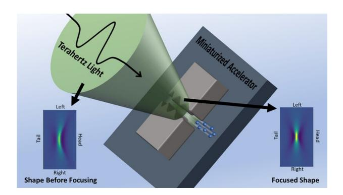
A pulse of terahertz light is focused (green) on a miniaturized particle accelerator to give energy to particles (blue spheres). New technology measures how the shape of the terahertz pulse (inset images) changes as it is focused on its target. Credit: Oak Ridge National Laboratory
