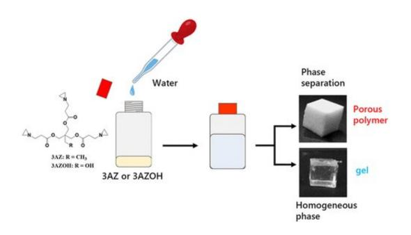
Researchers from SIT, Japan, discover that adding water to a triaziridine compound at mild temperatures is enough to produce strong and consistent porous polymers. By adjusting the reaction temperature and the initial triaziridine concentration, the morphological and mechanical characteristics of the polymers can be controlled. Credit: American Chemical Society.
