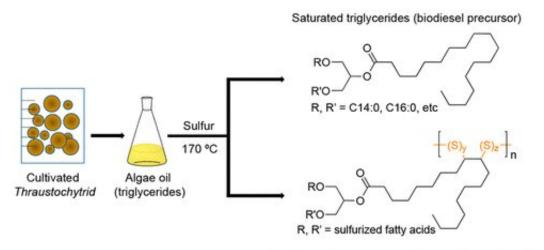
Copolymer from unsaturated triglycerides and sulfur (cathode material, metal sorbent, insulation, fertilizer)
