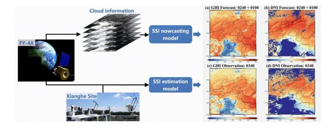
Schematic diagram of the Fengyun-4 geostationary satellite-based solar energy nowcasting system. Credit: Huang Chunlin
