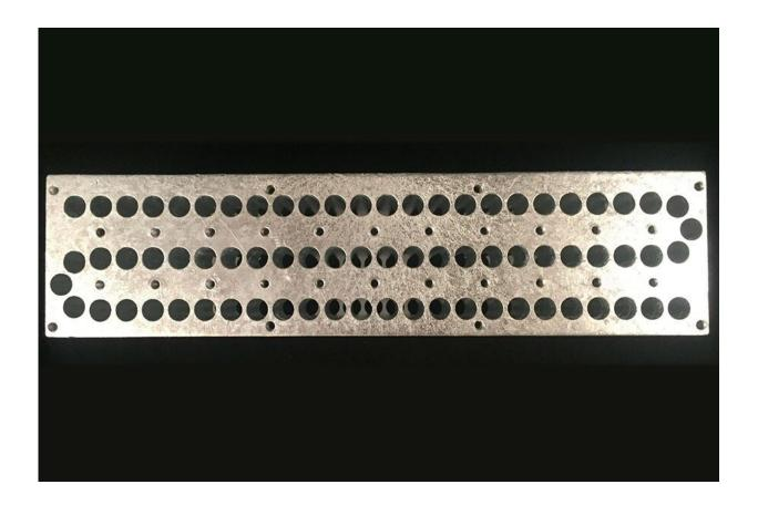
A new "quantum flute" experiment by University of Chicago physicists could point the way towards new quantum technology. The holes create different wavelengths, akin to 'notes' on a flute, that can be used to encode quantum information. Credit: Photo courtesy of the Schuster lab
