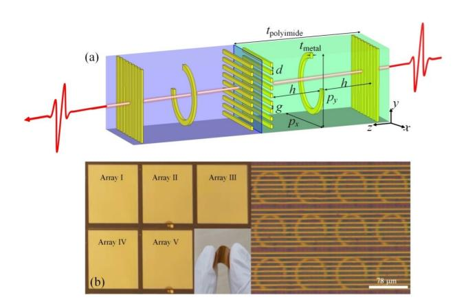
(a) Perspective view of the unit cell of array. (b) Overall and local optical images of the CEP shifter from top view, and flexibility of the CEP shifter demonstrated by manually bending the sample. Credit: AIR
