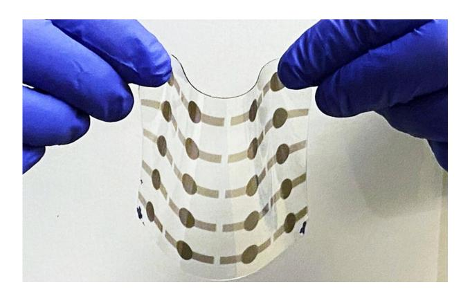
A 4x5-inch film made of 10 layers of processable, high-performance dielectric elastomers (PHDE) stacked together with 20 actuators. Credit: Soft Materials Research Lab/UCLA
