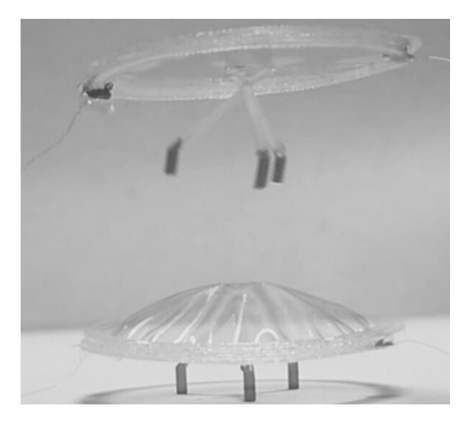
A jumping robot, about 1.2 centimeters in diameter, fitted with PHDE actuators. Credit: Soft Materials Research Lab/UCLA
