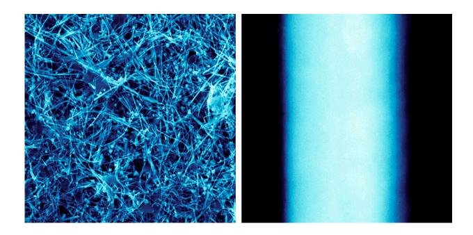
Left: Scanning electron microscopy image of the CuNW network on a coppersprayed surface. Right: Up-close image of CuNW nanowire, which is about 60 nm in diameter, approximately 100x smaller than a human hair. Credit: U.S. Department of Energy Ames National Laboratory
