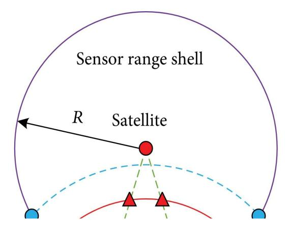
Geometry of dual-altitude band ATH coverage for a single satellite, shaded area. Credit: *Space: Science & Technology*
