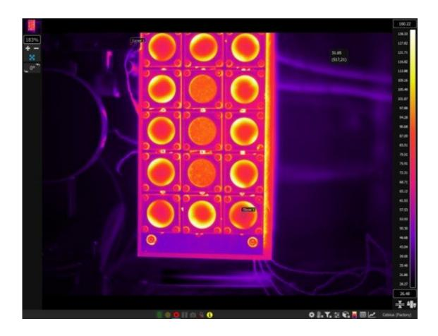
EnVision candidate materials sample observed by infrared camera. The samples are also heated as they are exposed to atomic oxygen by the LEOX generator to better simulate aerobraking through the atmosphere of Venus. Credit: ESA
