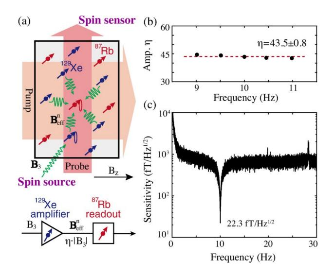
Magnetic-field amplification of the spin sensor. (a) Principle of using the spin sensor to search for exotic interactions. The signal from the pseudomagnetic field is enhanced by the <sup>129</sup>Xe-based amplifier, generating an effective magnetic field  $B_{eff}$  read out by <sup>87</sup>Rb spins. (b) The amplification factor 43.5±0.8 is
