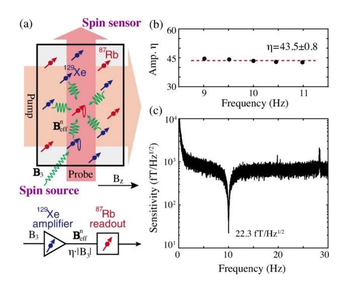
Magnetic-field amplification of the spin sensor. (a) Principle of using the spin sensor to search for exotic interactions. The signal from the pseudomagnetic field is enhanced by the  $^{129}$ Xe-based amplifier, generating an effective magnetic field  $B_{eff}$  read out by  $^{87}$ Rb spins. (b) The amplification factor 43.5±0.8 is
