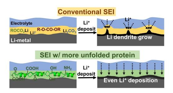
At the elevated temperature after protein-contained-electrolyte filling, the protein forms a functional-group-rich SEI on Li anode, building an even Li<sup>+</sup> deposition during cycling. Credit: Journal of Energy Chemistry
