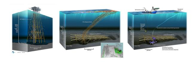
Illustrations of how the Taylor MC20 Platform in the Gulf of Mexico appeared before and after damage from Hurricane Ivan in 2004. The third panel shows the containment system installed to capture oil from persistent leaks. (September 2019 - Gulf of Mexico). Credit: NOAA/Kate Sweeney
