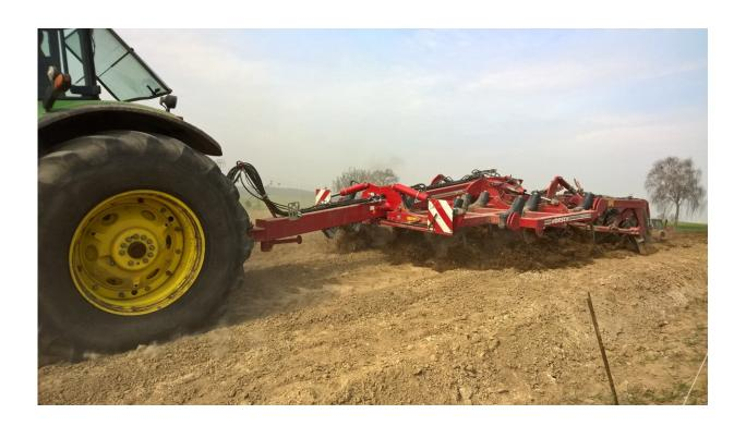
Soil tillage equipment moves large amount of material down slope as it is pulled through the soil' Credit: Professor John Quinton
