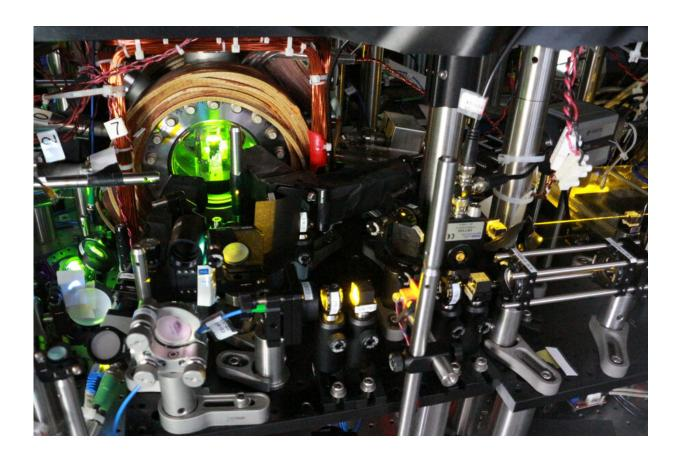
MIT researchers used a system of lasers to first entangle, then reverse the evolution of a cloud of ultracold atoms. Credit: Simone Colombo
