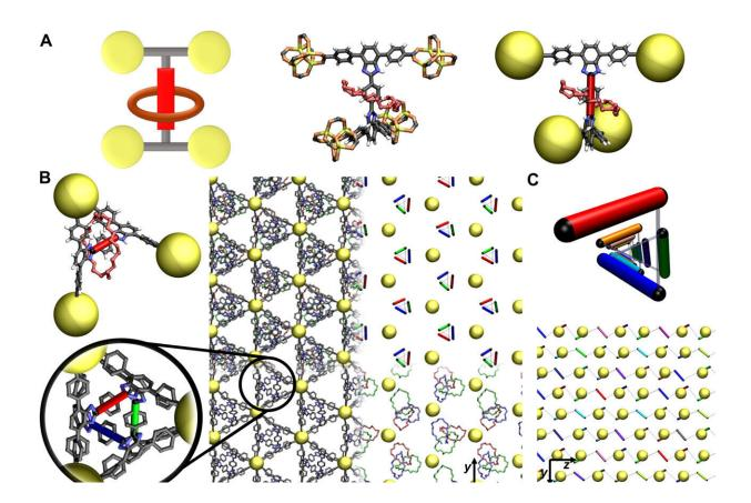
Molecular structure of the rotaxane functionalized MOF.(A) Representation of one organic linker connecting four inorganic  $Zn_4O$  corners. The left image sketches the structure of the building block, the center image shows an atomistic picture of the building block in ball-and-stick representation, and the right image shows a simplification of the atomistic picture. The inorganic corners are visualized by big yellow balls and the molecular crossbar (rotaxane axle) is
