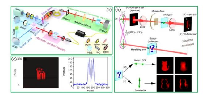
Fig. 3 Quantum switchable edge detection based on the photonic SHE in dielectric metasurfaces. (a) Experimental setup; (b) The first row is the illustration of coincidence measurement, and the second row shows the schematic of controlling the mode of quantum edge detection; (c) The edge detection image exhibits a high signal-to-noise ratio. Credit: Compuscript Ltd
