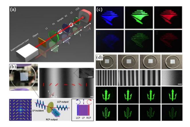
Fig. 2 Broadband image edge detection based on the photonic SHE in dielectric metasurfaces. (a) Experimental setup; (b) Sample of metasurfaces and illustration of edge detection; (c) Results of broadband image edge detection at different illumination wavelengths; (d) Results of image edge detection using metasurfaces with different periods. Credit: Compuscript Ltd
