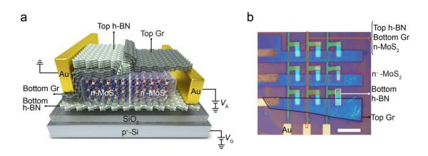
a. Schematic of a photon-controlled diode fabricated by sandwiching a h-BN layer between a  $n/n^-$  MoS<sub>2</sub> junction and a SiO<sub>2</sub>/p<sup>+</sup>-Si back-gate, using bottom/top graphene as cathode/anode and a top h-BN as protecting mask. b. Optical photograph of the fabricated array using photon-controlled diode as a unit. (scale bar: 10 µm). Credit: Science China Press
