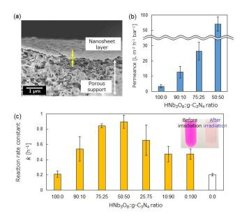
Figure 1. (a) Electron microscope image showing a cross-section of the nanosheet-laminated photocatalytic membrane developed in this study. (b) Comparison of how different combinations of nanosheets affect water permeation speed. (c) Changes in the rate constant of the rhodamine B photodegradation reaction depending on the combination of nanosheets (inset: photos showing the dye solution before and after photoirradition). Credit: Kobe University
