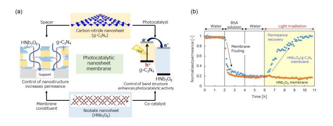
Figure 2. (a) The design of the novel nanosheet-laminated photocatalytic membrane, which uses two types of nanosheet, each with different functions. (b) Changes in the relative water permeation speed of the photocatalytic membrane before and after photoirradiation. Bovine serum albumin (BSA) was used as the
