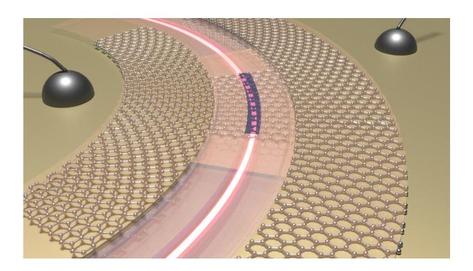
An artistic rendering of a silicon-based switch that manipulates light through the use of phase-change material (dark blue segment) and graphene heater (honeycomb lattice). Credit: Zhuoran Fang
