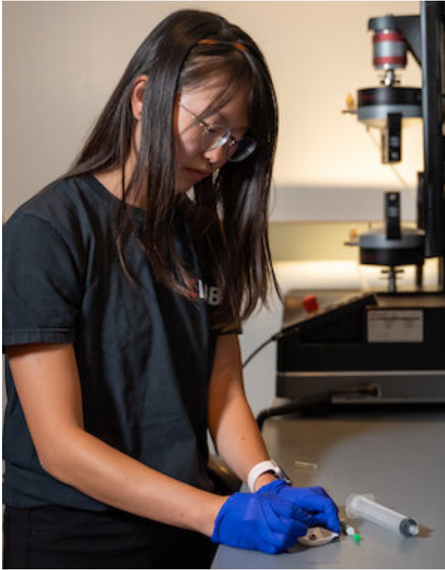
Rice graduate student Faye Yap with a deceased wolf spider. Yap attaches the spiders to a needle and feeds air into their limbs to act as a necrobolic gripper. Credit: Brandon Martin
