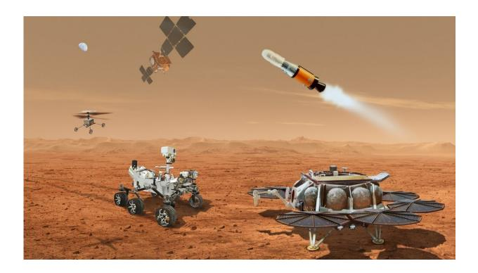
This illustration shows a concept for multiple robots that would team up to ferry to Earth samples of rock and soil collected from the Martian surface by NASA's Mars Perseverance rover. Credit: NASA/JPL-Caltech
