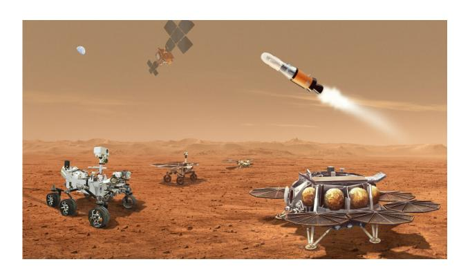
This illustration shows a concept for multiple robots that would team up to ferry to Earth samples collected from the Mars surface by NASA's Mars Perseverance rover. Credit: NASA/ESA/JPL-Caltech
