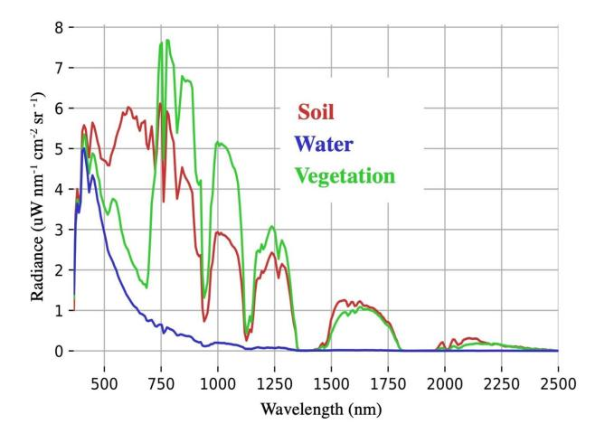
The line graph shows spectral fingerprints for soil, vegetation, and a river. Radiance indicates the amount of each wavelength of light (in nanometers) reflected from a substance. Credit: NASA/JPL-Caltech
