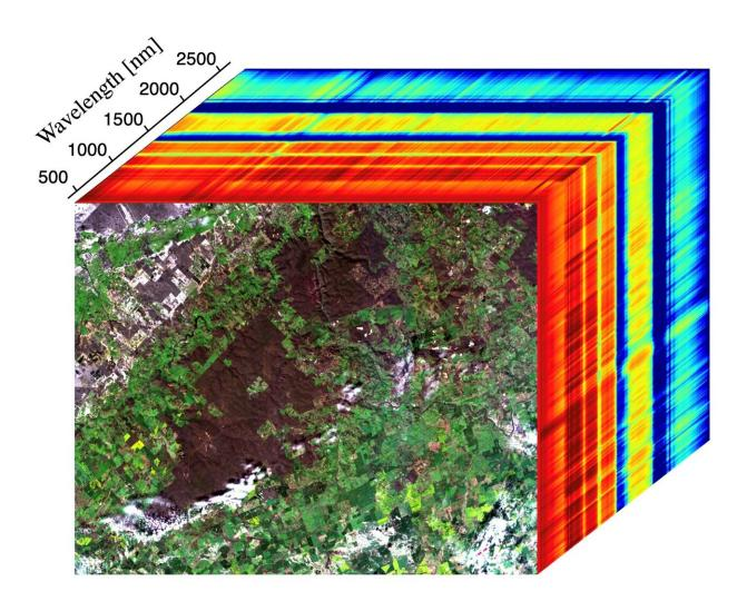
This image shows the first measurements taken by EMIT on July 27, 2022, as it passed over Western Australia. The image at the front of the cube shows a mix of materials in Western Australia, including exposed soil (brown), vegetation (dark green), agricultural fields (light green), a small river, and clouds. The
