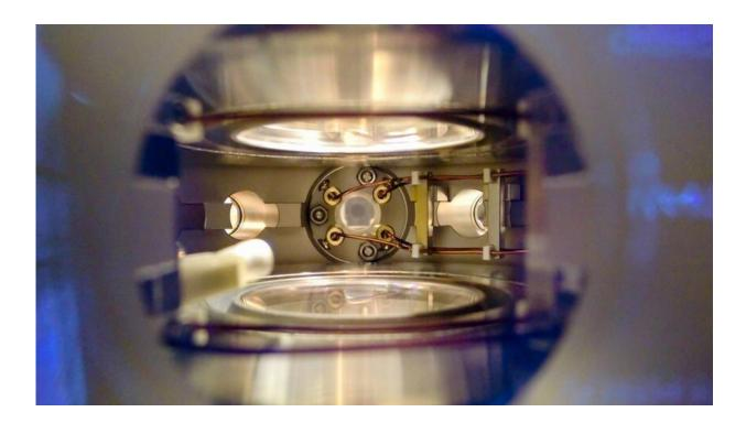
A close view inside the main vacuum chamber of the NaK molecules experiment. In the middle four high-voltage copper wires are routed to an ultrahigh-vacuum glasscell where the ultracold polar molecules were produced. Credit: Max Planck Society
