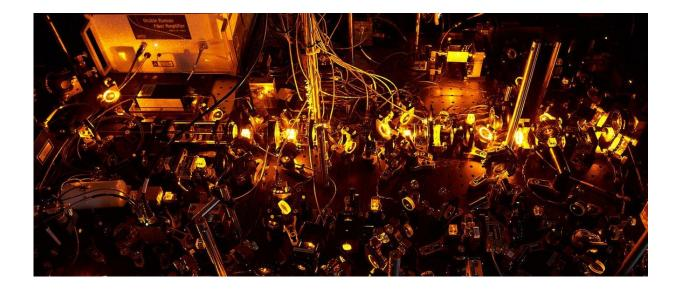
Picture of the sodium laser system generating the yellow light used for laser cooling and imaging of sodium atoms. Credit: Max Planck Society
