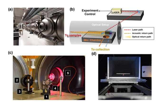
The system is based on a beam of light and captures the emission of the elements that make up the sample and, at the same time, the acoustic wave produced in the detonation of the mineral. Credit: *Analytical Chemistry* (2022). DOI: 10.1021/acs.analchem.1c04792
