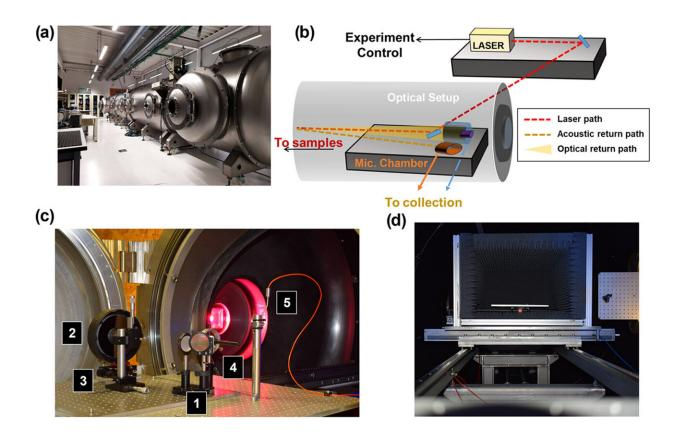
The system is based on a beam of light and captures the emission of the elements that make up the sample and, at the same time, the acoustic wave produced in the detonation of the mineral. Credit: *Analytical Chemistry* (2022). DOI: 10.1021/acs.analchem.1c04792
